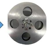
Like most Fe-based materials, Nanocrystalline tends to oxidise after exposure to atmosphere. Therefore, after opening the product from its packaging, it is to be used as soon as possible to avoid deterioration from exposure to climatic conditions.
