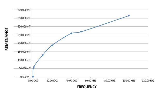
Source: HIGH FREQUENCY MAGNETIC ANALYZER
